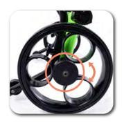
Adjustable resistance helps control speed. Ideal for beginners or users needing slower, safer movement. Reducing resistance allows for freer, more dynamic motion.
