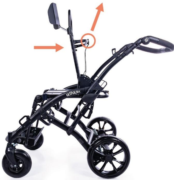
Pull the handle up and adjust the backrest angle
