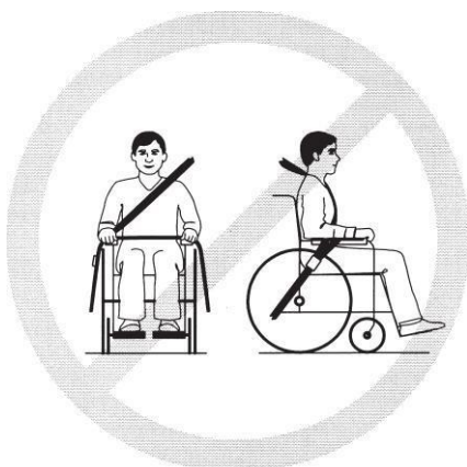
Fig. 20.7 Improper fit of the belt
