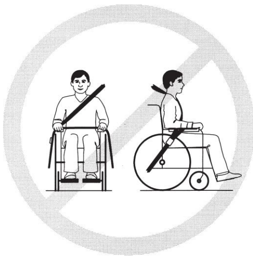
Fig 20.5.D Improper adjustment of belt
