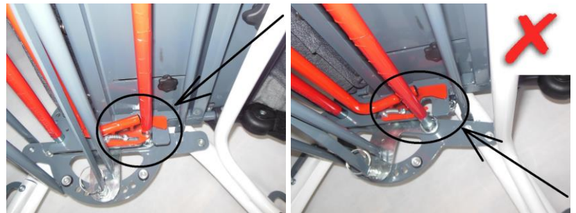
Fig..8.26.-F - CORRECT Fig..8.26.-F' – WARNING! WRONG!
