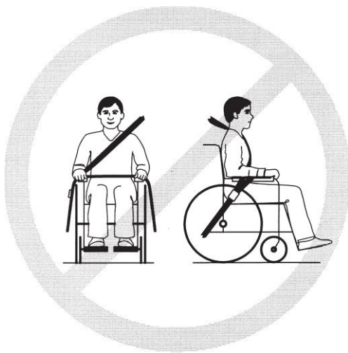
Fig 20.5.D Improper adjustment of belt
