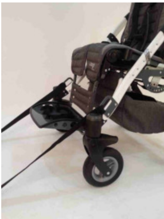
Figure 20.5.2. - Proper placement of fastening
